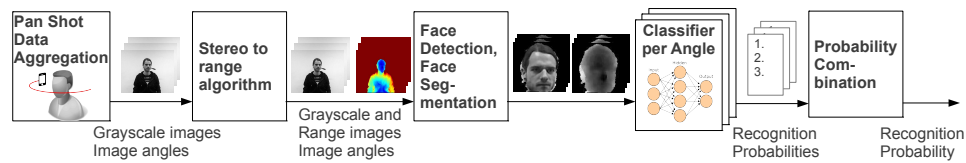
Figure 5.2: Overview of modules used in the stereo vision pan shot face unlock toolchain.
