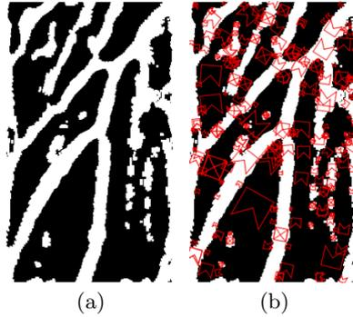
**Fig. 3.** Preprocessed vein pattern sample (a) and its extracted SIFT features (b).
