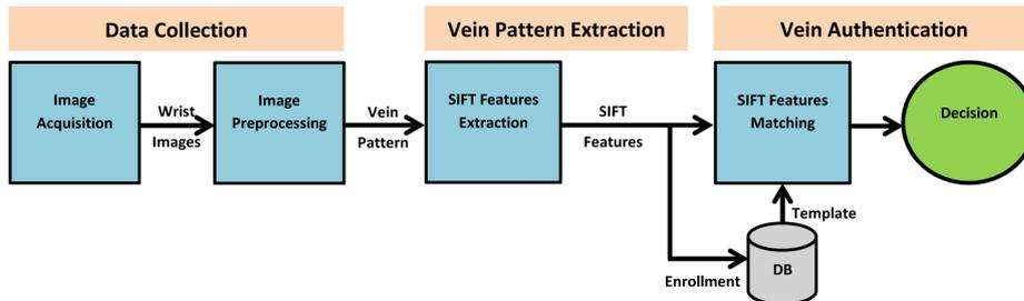
Fig. 1. Constituent parts of our approach to mobile vein pattern authentication.
