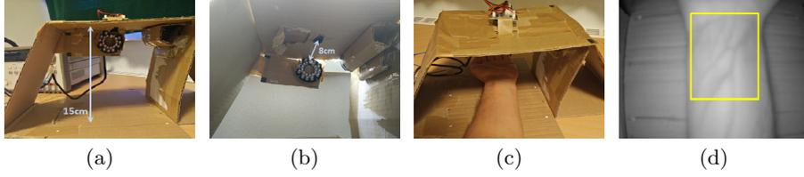
**Fig. 4.** Capturing device camera position (a), NIR LEDs position (b), hand position (c), camera view with ROI (d).
