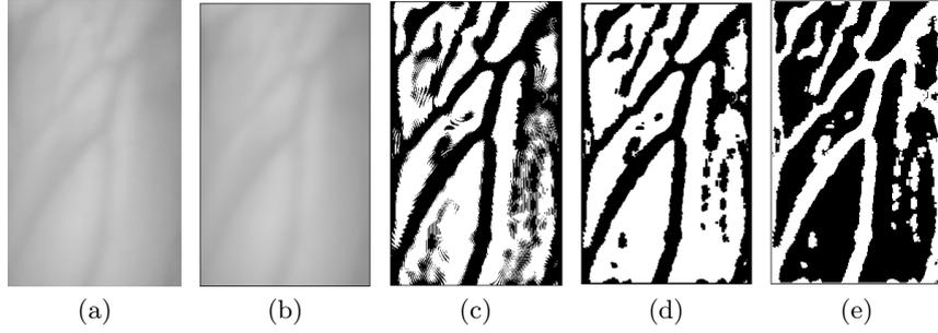
**Fig. 2.** Vein image preprocessing: sample after applying cropping (a), filtering (b), auto local threshold (c), morphological closing (d), and pixel inversion (e).
