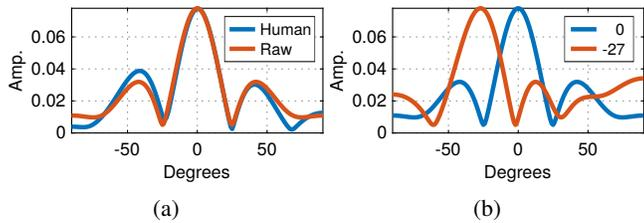
FIGURE 4: (a) Comparison of the amplitude of the array response  $|\mathbf{a}_{hf}(\mathbf{t})|$  when environment is human-free vs  $|\mathbf{a}_{hp}(\mathbf{t})|$  where a human exists at  $-27^\circ$  at a particular time instant. (b) Amplitude of the modeled array response  $|\hat{\mathbf{a}}_j|$  for a unit source impinging on the ULA from directions  $\theta = 0^\circ$  and  $-27^\circ$ .
