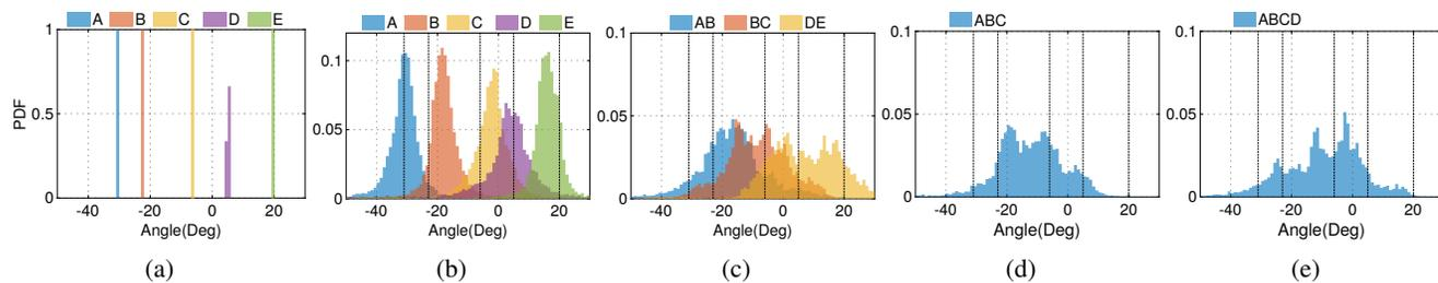
FIGURE 9: Direction of arrival distribution in different scenarios. (a) No human exists, a TX is placed at A, B, C, D & E in separate measurement campaigns, (b) one human exists at A, B, C, D & E in separate measurement campaigns, (c) two humans exist at AB, BC or DE within 0.5 m in three separate measurement campaigns, (d) three humans exist at ABC 0.5 m from each other and (e) four humans exist at ABCD 0.5 m from each other.
