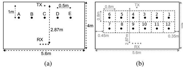
FIGURE 5: Experiment Environment. # of RX antennas: 4, # of TX antennas: 1, antenna heights from ground: RX 0.89 m, TX 0.85 m, room size: 5.6 m  $\times$  4 m  $\times$  2.184 m. (a) A to E and (b) 1 to 12 are anchor points.
