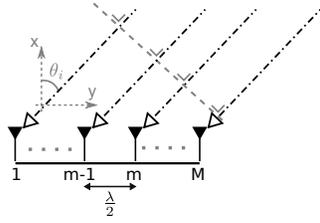
FIGURE 1: A plane wave impinging on a antenna array at an azimuth angle of  $\theta_i$ .
