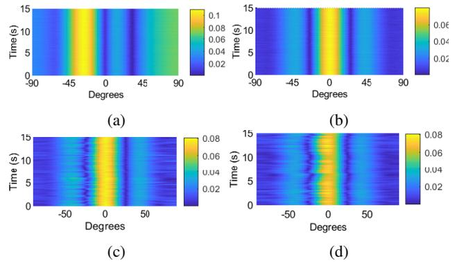
FIGURE 2: (a) Array response for a signal emitted from anchor point A at  $-28^\circ$  during 15 s and array response when a signal is emitted from C at  $0^\circ$  (b) no human exists in the environment (c) a human exists at A and (d) a human exists at A and at B.
